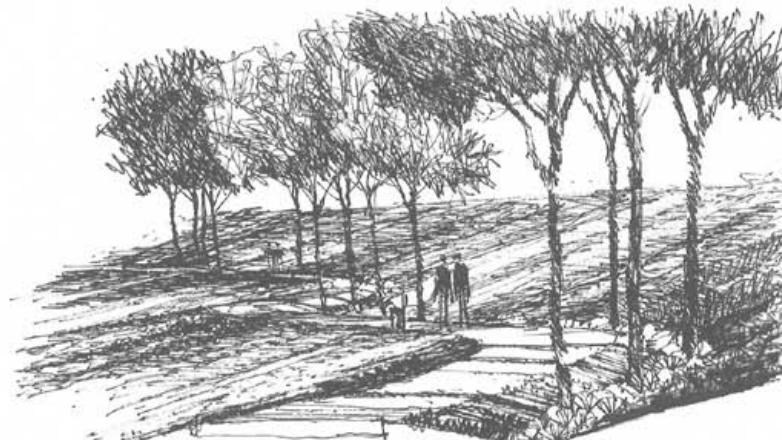
**Drainage Corridor Illustration:** A network of drainage corridors will connect developed neighborhoods to Westerly Creek and other primary drainageways, serving to detain water and clean pollutants from the urban runoff. As stormwater infiltrates along the canal, it will sustain a network of trees and vegetation. A pedestrian path will allow access for periodic maintenance and cleaning.
