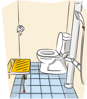
After: Installation of foldable shower seat against the wall.
