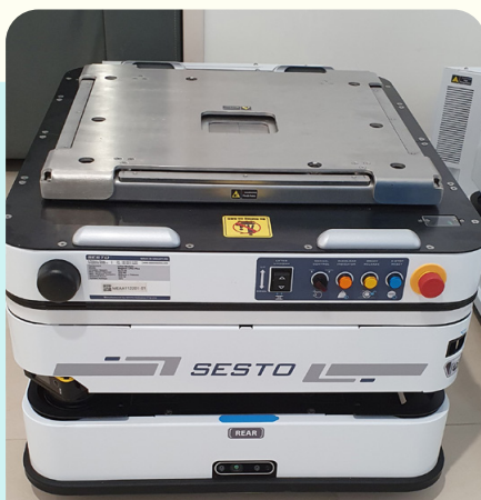
AMR to lift and transport trolley containing meals, laundry or consumables
