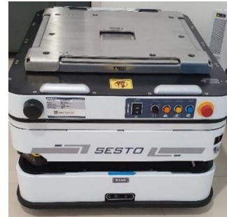
AMR to lift and transport trolley containing meals, laundry or consumables
