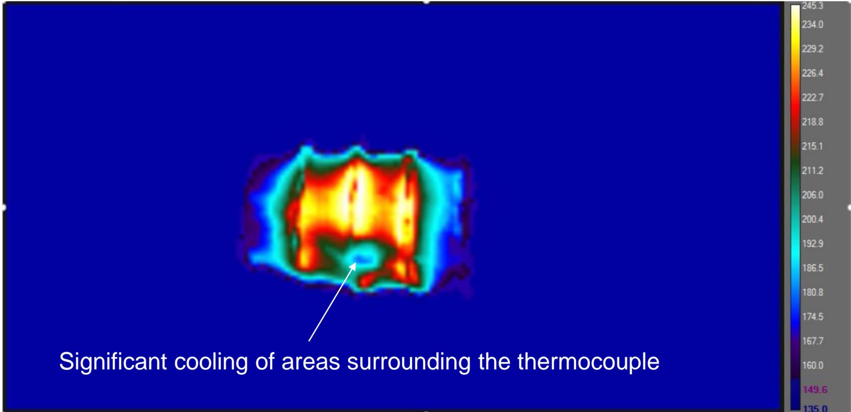
Significant cooling of areas surrounding the thermocouple
