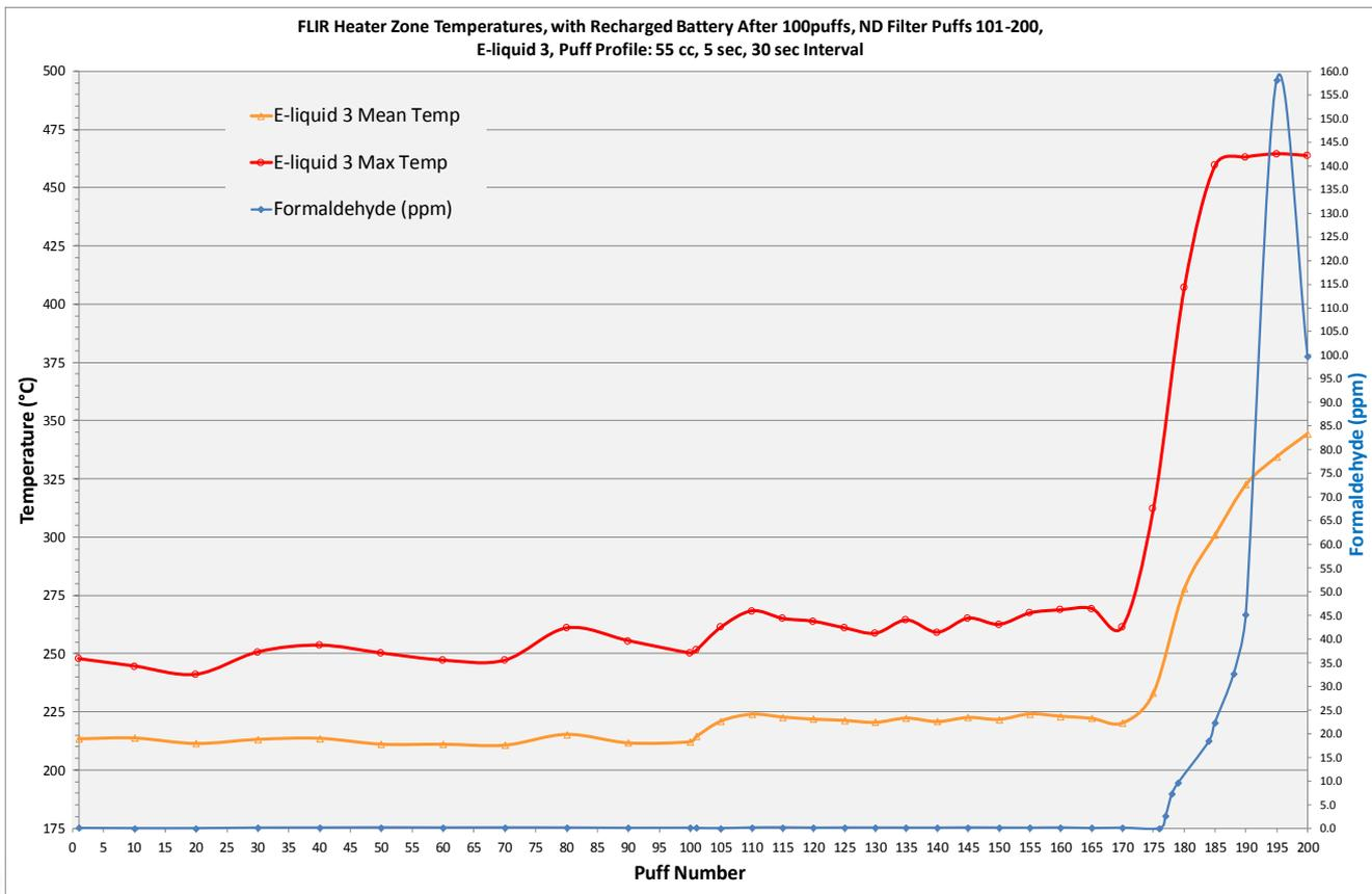
In this example, Formaldehyde begins to evolve between 350-400°C, using B1 battery.
