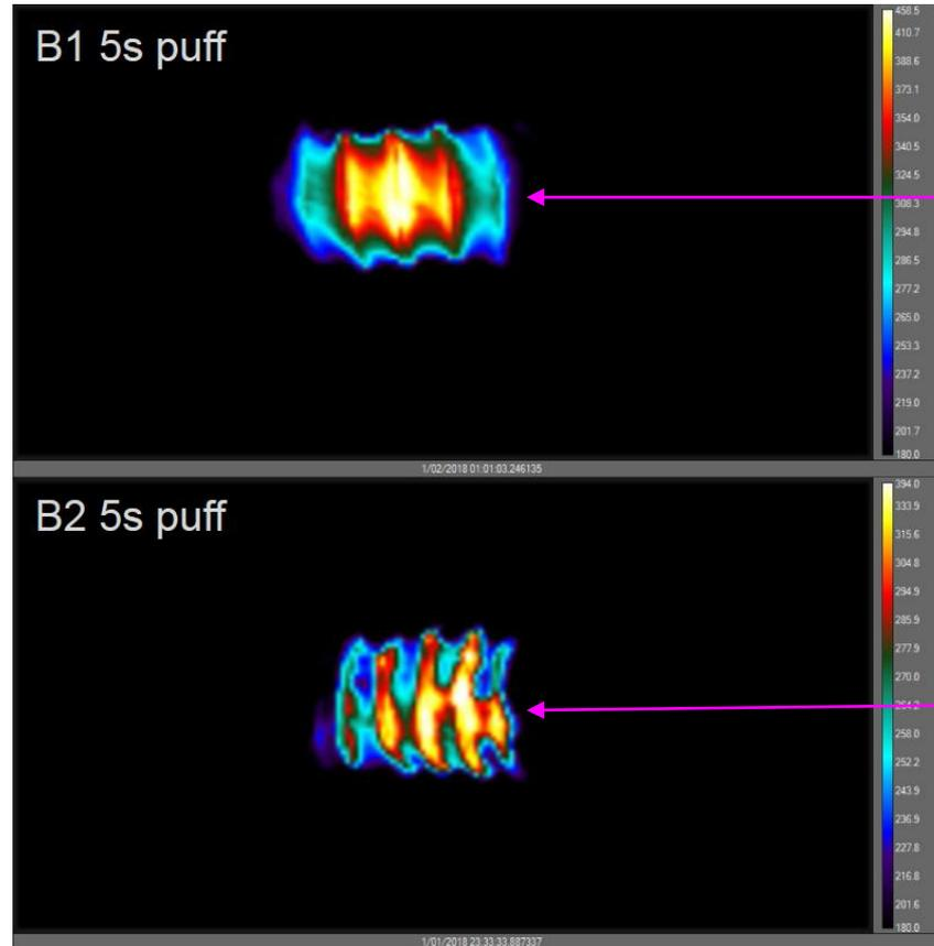
No cutoff B1 battery, captured image near the end of the 5s puff
