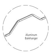
SkyWrap cable is passed around the tower top conductor fittings using a specially designed bypass accessory known as a "balehanger." The aluminum balehanger is clamped to the conductor either side of the conductor fittings and the SkyWrap cable is secured within a channel holding it in position away from the conductor fittings.
