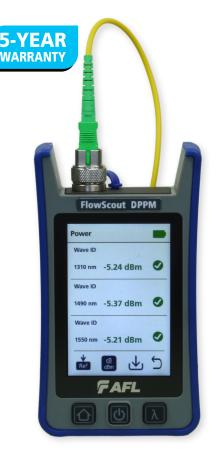
AFL's FlowScout Downstream PON Power Meter (DPPM) is designed to automatically detect and simultaneously measure coexistent downstream PON power levels at 1490 nm GPON/EPON and either 1550 nm RF video or 1577 nm XG/XGS/10GEPON.
