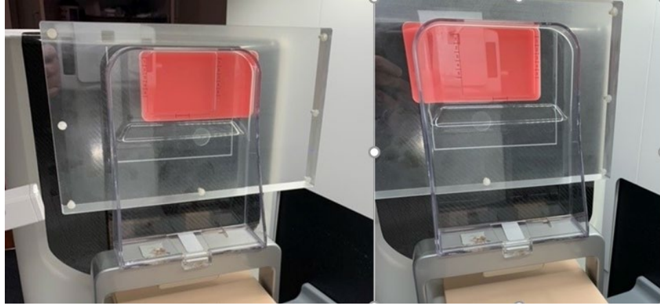
323 324 Figure 2-3: Showing that the ACR DM Phantom was imaged twice to make sure all test 325 objects could be visualized inside the view window.
