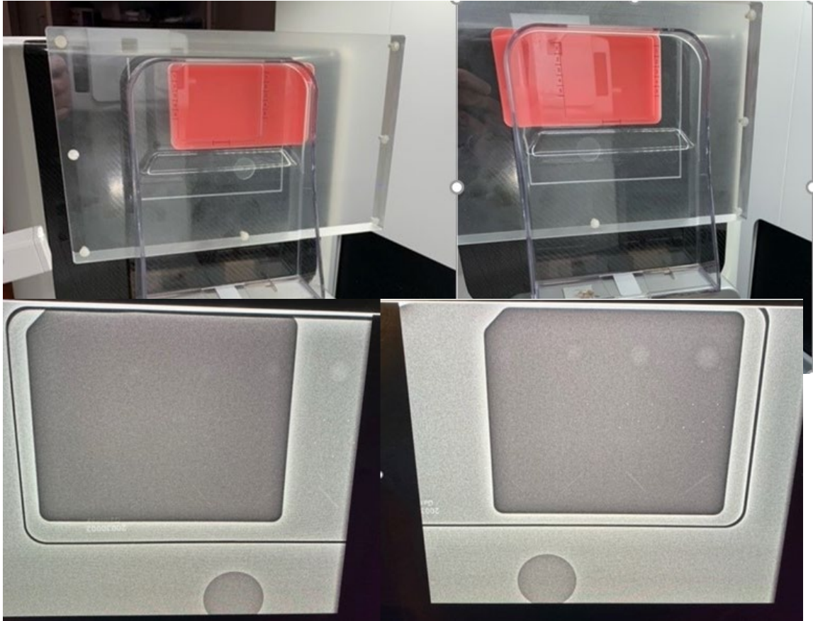
Figure 3-3: ACR DM phantom imaged twice to make sure all test objects could be visualized inside the view window.
