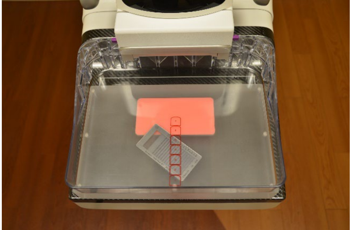
Figure 3-6: Bar pattern placement for the Spatial Resolution test on a 2D system. The bar pattern is at a 45° angle to the chest-wall edge.
