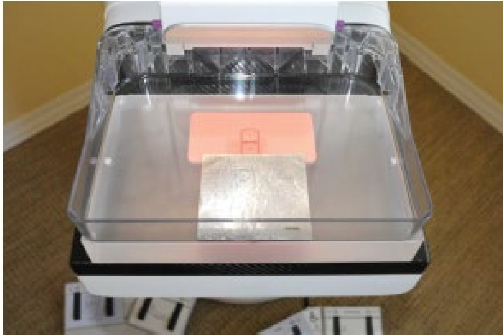
1484 Figure 3-14. Note coverage of image receptor and placement of aluminum
