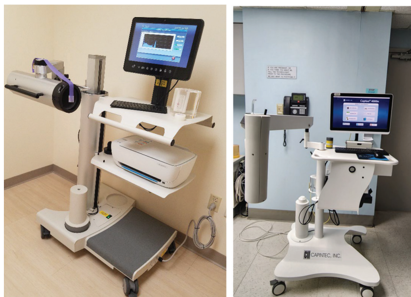
Figure 4-14. Quality control configurations for two different types of commercial uptake probes.
