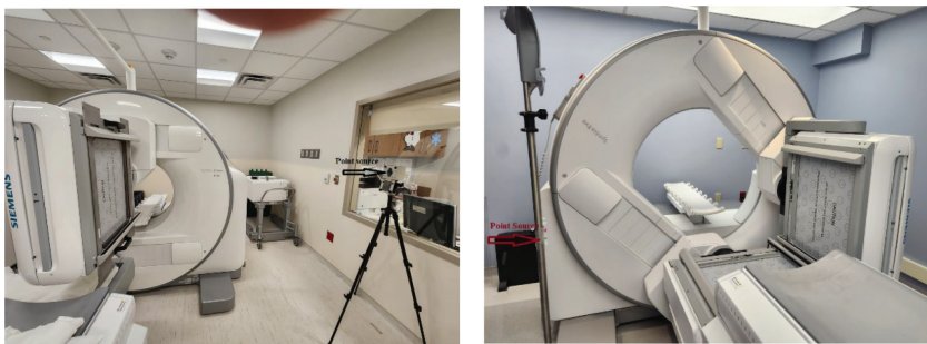
Figure 4-7. Setup for count rate measurement with point source attached to a tripod (left) or pole (right) placed at a height centered with the detector.
