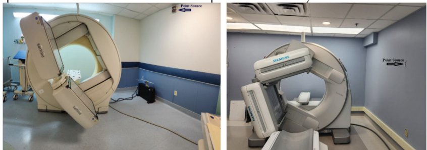
Figure 4-2. Two different detector configurations for intrinsic uniformity for dual-head gamma cameras. The point source must be at a distance of 3 to 5 UFOV. The system on the left acquires both detectors simultaneously, whereas the system on the right acquires one detector at a time.
