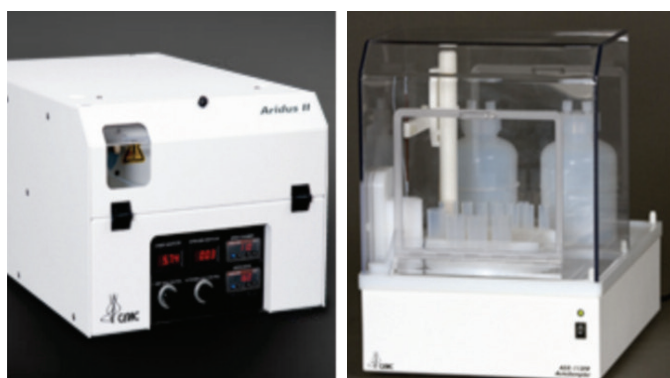
Figure 2: Sample introduction system used for the dry plasma experiment (Cetac Aridus II, left) and autosampler used for all measurements (Cetac ASX112, right).
