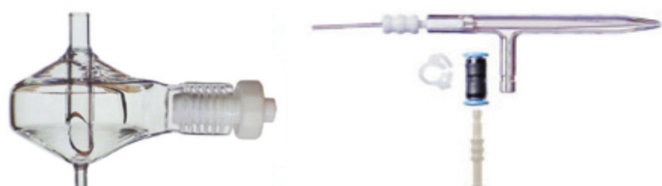
Figure 1: Wet plasma sample introduction system consisting of baffled cyclonic spray chamber and microconcentric nebuliser, both manufactured by Glass Expansion.
