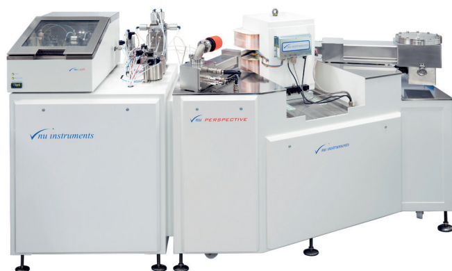
Figure 1: Nu carb with dual inlet and adsorption trap
