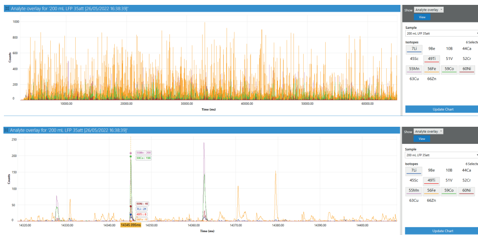
Figure 3: Upper figure shows the nanoparticle signals of lithium battery electrode materials captured over 40 seconds using the gravitational counter flow device. The lower image is a zoomed section (14.32s – 14.39s) showing the traces for individual particles collected with 80 \mu s spectra.
