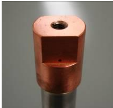
Figure 3-7. ¼-20 Threaded Hole in the Cold Tip
