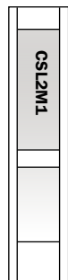
2 3/4" stiles, 6 1/2" top rail & 12" bottom rail with 5 5/16" intermediate rail 35" from bottom of panel
