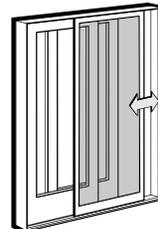
Patented square corner joint construction adds considerable strength to the frame members. The insect screen is available for both two-panel doors and four-panel doors. Gliding insect screens have Delrin® injection-molded bottom rollers with self-contained leveling adjusters, providing smooth operation. Interior and exterior pulls and latch are provided.
