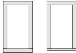
Flat casing can be used on all four sides flush at the head and sill. Combine 3 1/2" (89) and 4 1/2" (114) flat casing or use with a flush sill nose.
