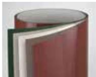
Factory-finished in any of our 11 exterior trim colors, our aluminum coil stock allows you to form your own profiles in the field. Made from .018" thick aluminum, coil stock is available in 24" (610) x 50' (15240) rolls. Color-matched stainless steel trim nails are also available and can be ordered in 1 lb/.454 kg boxes.
