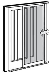
Patented square corner joint construction adds considerable strength to the frame members. The insect screen is available for both two-panel doors and four-panel doors. Gliding insect screens have Delrin® injection-molded bottom rollers with self-contained leveling adjusters, providing smooth operation. Interior and exterior pulls and latch are provided.
