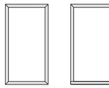
Brick mould can be used on all four sides or with a flush sill nose.
