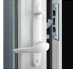
Hook deadbolt lock comes pre-installed, reducing installation time. The mortised lock and hook design provides strength and added security compared to bored locks with standard deadbolts. Multi-point locks are standard on 7'-6" (2286) and 8'-0" (2438) height doors. Multi-point locks can be ordered for 6'-8" (2032) and 6'-11" (2108) doors as an option. Contact your Andersen supplier for availability.
