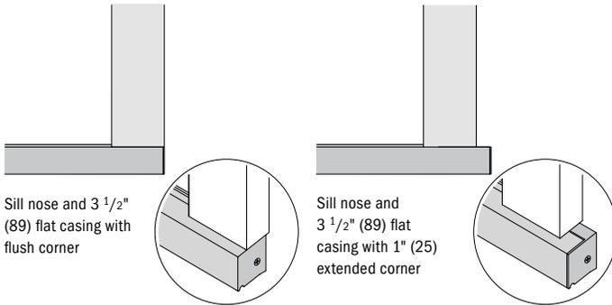
Sill nose and 3 1/2" (89) flat casing with flush corner
