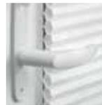
Extends interior door handle an additional 1" (25) from the door panel to accommodate interior blinds or shades. Kit includes one handle extender and spindle. A second extender may be added to the spindle to increase the length an additional 1" (25) to a 2" (51) total extension. Extenders are available in finishes that coordinate with hardware.
