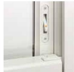
A recessed window opening control device is available factory applied. It limits the sash travel to less than 4" (102) when the window is first opened. Available in stone and white. A field-applied window opening control device is also available.
