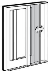
The retractable insect screen is installed on the exterior of the door and opens side to side across the width of the opening. When the insect screen is not in use, it neatly retracts into a small canister mounted on the exterior of the door. The retractable insect screen canister is available for two-panel patio doors in our six standard exterior colors. Please note, retractable insect screen track reduces clear opening height by 1" (25)
