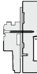
Available in 8'-0 1/4" (2445), 9'-6" (2896) and 12'-6" (3810) lengths. Treated for corrosion resistance, the material has a 4" (102) depth that provides strength and rigidity. Adjacent windows attach to the steel joining with screws provided in the kit. Use with windows and patio doors. 200 Series Perma-Shield® gliding patio door is shown above with a 400 Series casement window.
