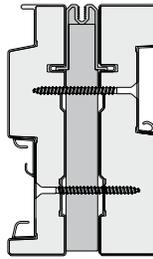
Laminated Veneer Lumber (LVL) joining material is available for gliding patio doors. Both 4 9/16" (116) x 3/4" (19) LVL and 6 9/16" (167) x 3/4" (19) LVL are available and include an aluminum exterior trim strip retainer. LVL materials are available in a variety of lengths up to 10' (3048).
