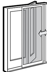
Available for two-panel active-stationary doors. Features Delrin® material injection molded bottom rollers with self-contained leveling adjusters.
