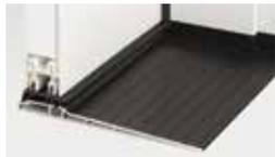
Andersen offers a single-panel accessible door that is 3'-2 1/8" (968) wide and includes a low-threshold sill [1/2" (51) high]. Bottom rail height is 10 1/4" (260). Available in bronze anodized finish only. Low threshold sill is not available for other door widths.
