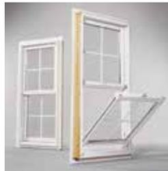
A convenient tilt-wash design makes it easy to clean the window from the inside. An in-sash balancer minimizes the view of the jamb liner, maximizing the amount of wood in the frame. Window can be secured through the side jambs to stud walls without hitting balancer.
