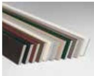
Andersen offers a 3 1/2" (89) wide by 3/4" (19) thick cellular Fibrex trim board in 10' (3048) lengths. Available in the same 11 colors as the exterior trim system, this solid trim board can be ripped to size and can be fastened using nails or screws.
