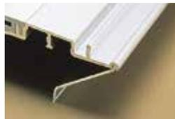
An aluminum sill support is designed to lock into a channel under the sill and tie back into the wall. This will offer support to the outermost sill section when needed. Available in neutral gray finish.
