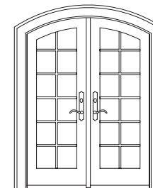
Auxiliary hinged patio door with arched top and flat trim with backband
