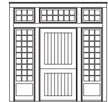
Dutch door main entry with substantially sized sidelights and transom windows
