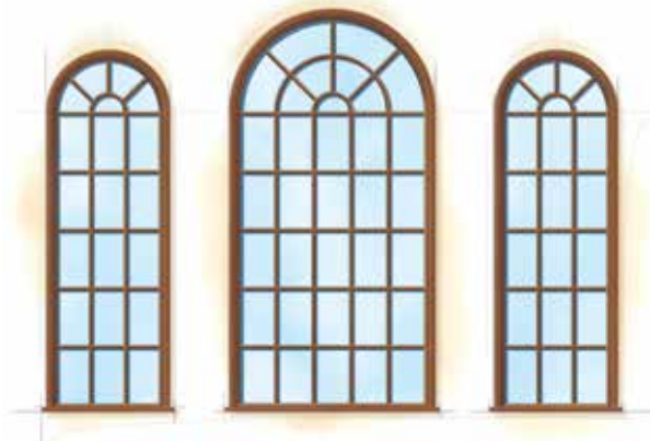
Auxiliary extended half circle window (interior)
