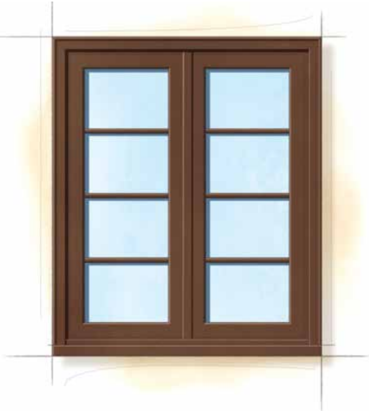
Exterior trim is often not used when windows are recessed into exterior wall veneer.
