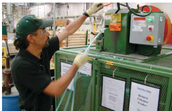
Milling Operator Mike Fehlen feeds a batch of plastic banding into a chopper.
