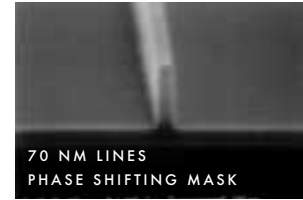
FIG. 10: RESIST PATTERNS IMAGED WITH AN ADVANCED LITHOGRAPHY SYSTEM. THE 130 NM LINE WHICH IS USED IN STATE-OF-THE-ART MANUFACTURING. THE 110 NM AND 70 NM LINE THAT SHOW THE CAPABILITY FOR FUTURE GENERATION OF DEVICES.
