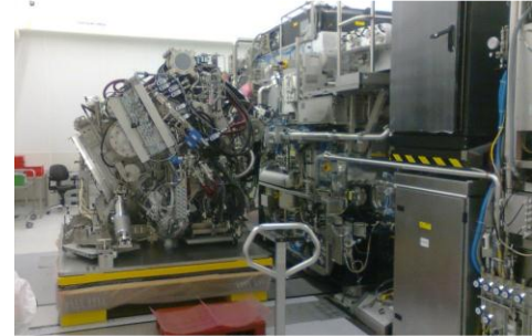
Pilot 2 reliability testing Ushio source installation
