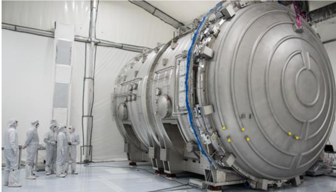
High NA optics metrology vessels installed in cleanroom @ Zeiss SMT
