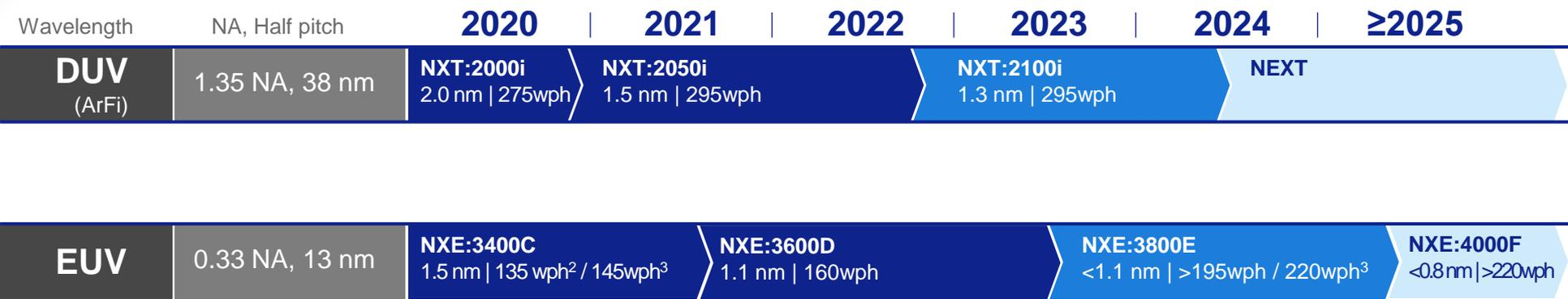
wafers/hours (wph) are based on 30mJ/cm<sup>2</sup>
