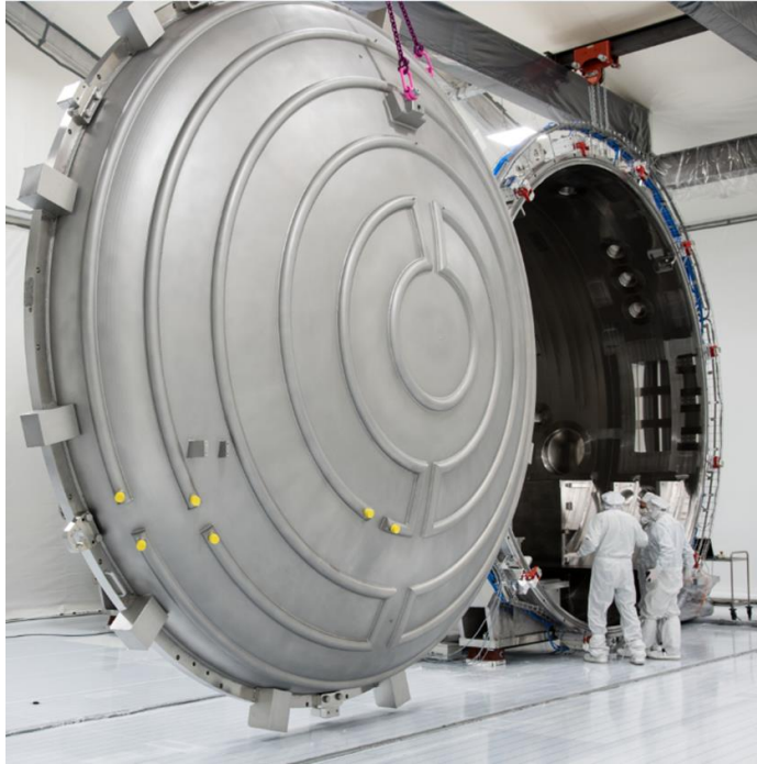
Optics metrology vessel installed in High NA cleanroom
