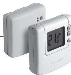
**GB** The RD-1200 wireless room thermostat comprises a RD-1200 Room Thermostat and a Relay Box. These devices communicate on an 868MHz Radio Frequency (RF) band to control a single heating system component such as a boiler, pump or zone valve. RF communication is 2-way, allowing high performance energy efficient control, display of boiler information, and easy setup and communications check features.
