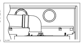
Fasten the suction pipes using two galvanised Ø 4,2 mm self tapping screws with minimum length 19 mm. If not included with the supply, screws with the same characteristics must be sourced on the market separately.
