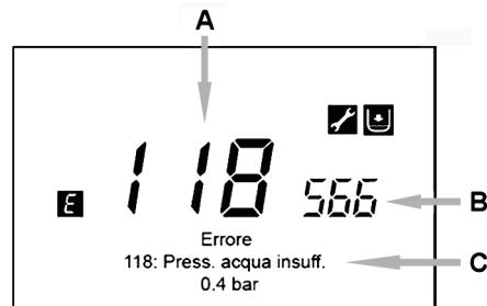
The faults shown on the display are identified with the symbol
