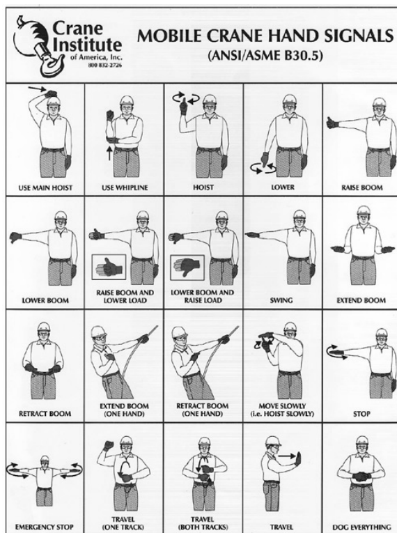
Figure 1 Mobile Crane Hand Signals ANSI/ ASME B30.5
