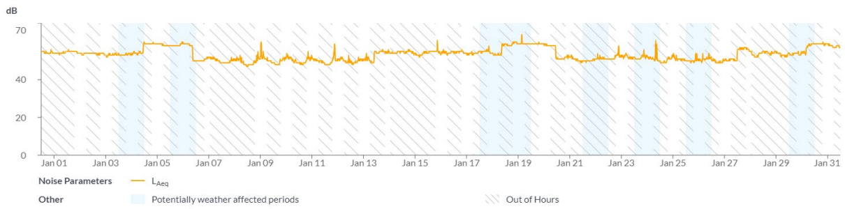
Figure 5 SiteHIVE noise monitoring data at EDR/AAR during January 2023
