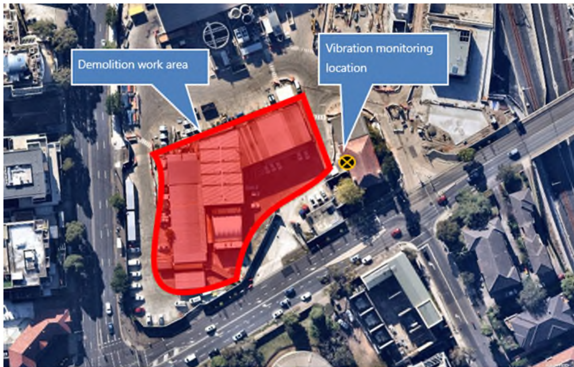
Figure 2.1: Vibration monitoring location
