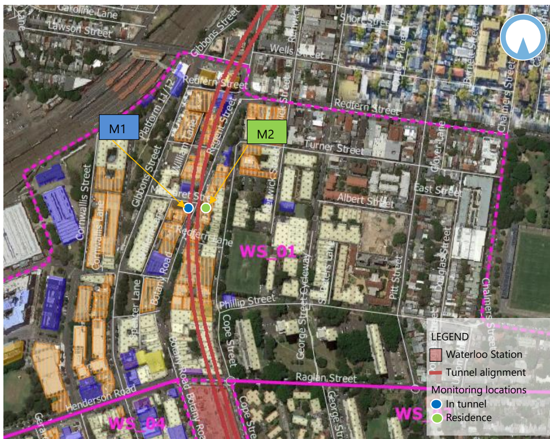
Figure 2-1 – Vibration monitoring locations at Waterloo-Central tunnel and residential receiver
