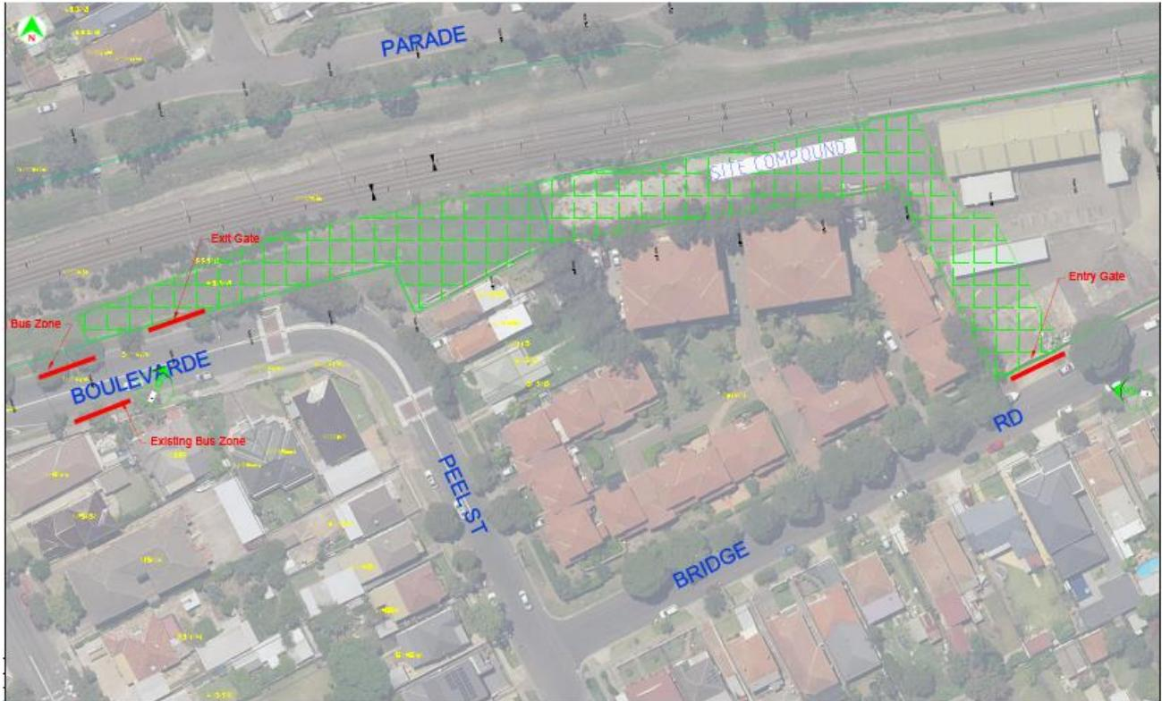
Figure 8. Temporary site office at Bridge St, Belmore (refer to Appendix A for details)
