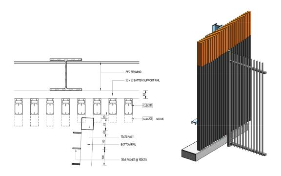
Figure 6-22 Chatswood Dive - Façade and fence junction detail - Plan (left and Isometric (right)
