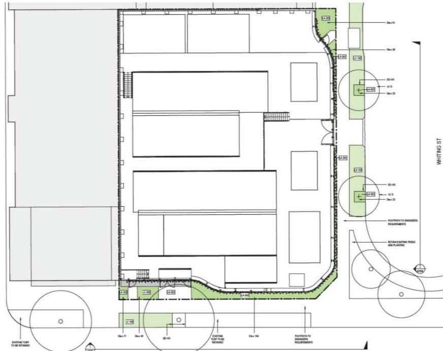
Figure 5-5 Artarmon Substation Landscape Plan
