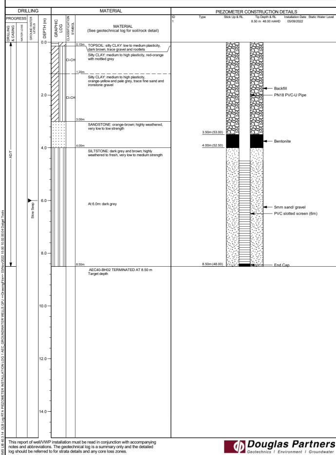
This report of well/VWP installation must be read in conjunction with accompanying notes and abbreviations. The geotechnical log is a summary only and the detailed log should be referred to for strata details and any core loss zones.
