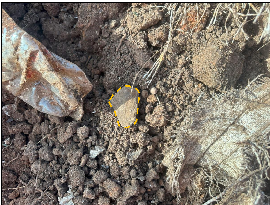
Site Photograph 4: Representative asbestos fibre cement fragment encountered within the stockpiled material, as observed 24 May 2024.
