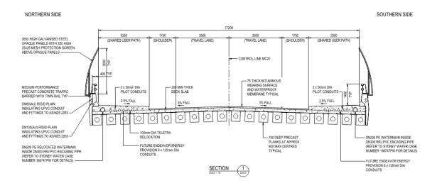
Figure 19: Proposed cross section on Lansdowne Road bridge during traffic stage 3
