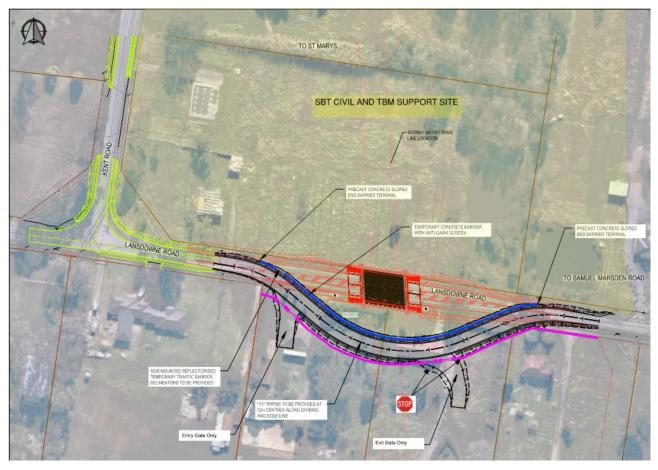
Figure 14: Proposed site access/egress gates on Lansdowne Road during Traffic Stage 2 (indicative purpose only)
