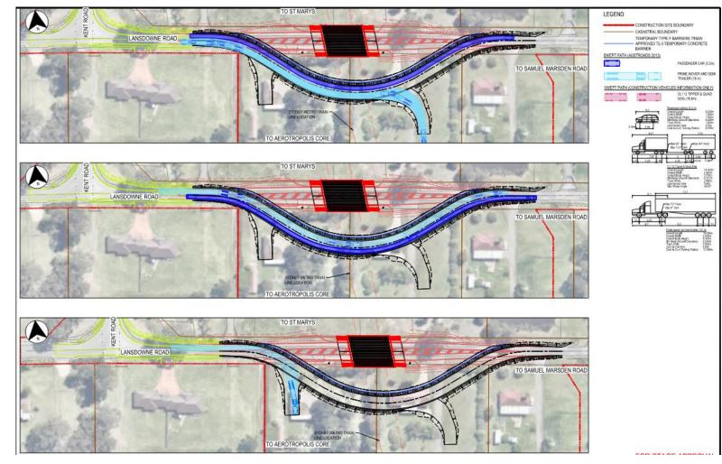
Figure 17: Swept path on side-track during Traffic Stage 2
