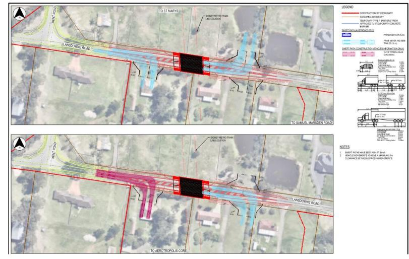
Figure 20: Swept path on Lansdowne Road bridge during traffic stage 3
