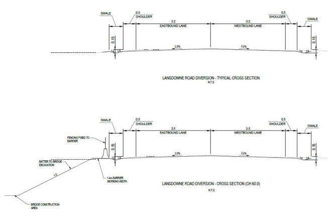
Figure 16: Proposed cross section of side-track during traffic stage 2
