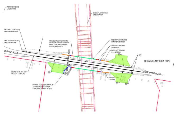
Figure 18: Proposed site access/egress gate on Lansdowne Road during Traffic Stage 3 (indicative purpose only)
