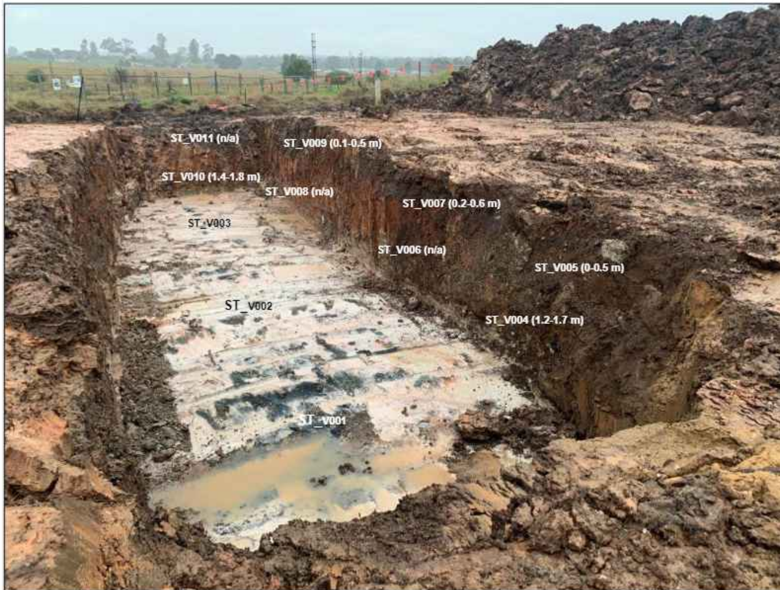
Photograph 1 – North and east wall partial base (base samples 2.4 m) (n/a – not analysed)
