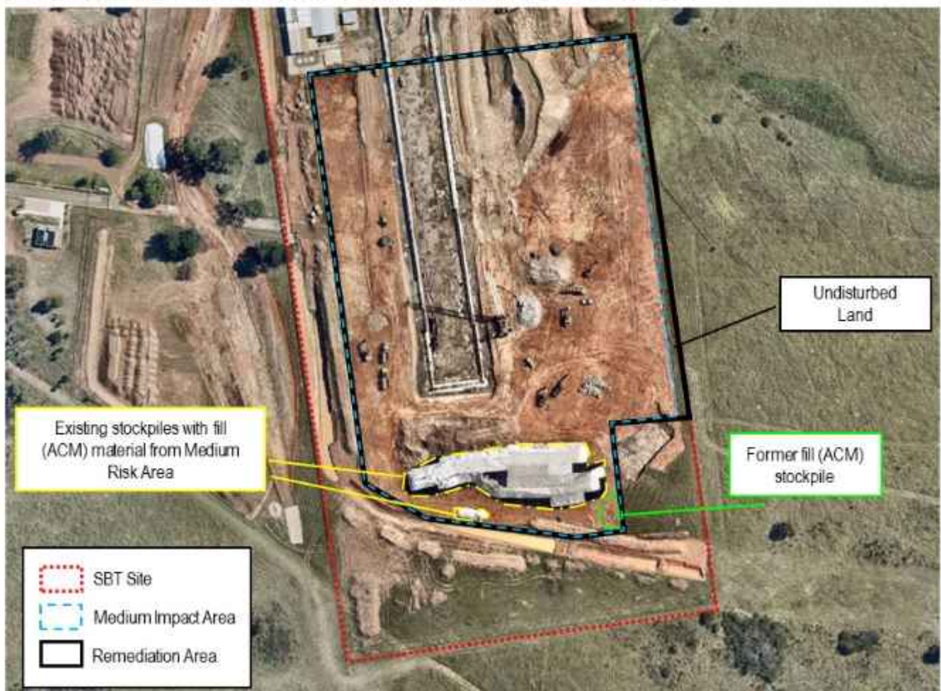
Figure E Existing Site Conditions
