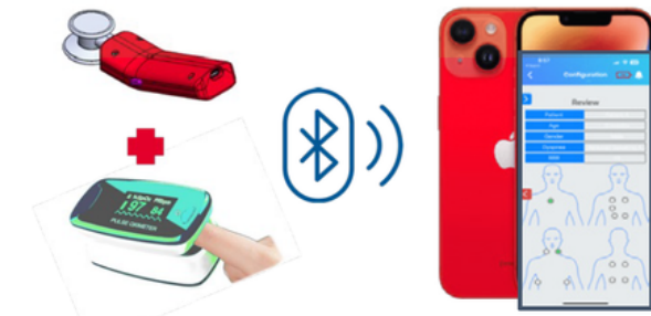
StethAid Lungs consists of a digital stethoscope, mobile app, website portals, and cloud storage. StethAid Lungs combined with oximeter was used to build asthma lung sound database.
