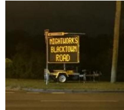
Consider the use of traffic Variable Message Signs (VMS) as an additional communication tool to notify the community of upcoming out of hours works.
