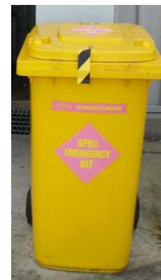
Spill kits are located at all Endeavour Energy FSC's and substations and should always be easily accessible
