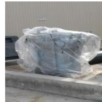
Wrapping a transformer before transport
