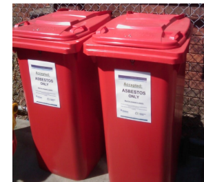
For Endeavour Energy employees, dedicated bins for asbestos disposal (bonded and asbestos PPE only) are available in all FSCs. Asbestos waste must be double wrapped and sealed with asbestos warning labels
