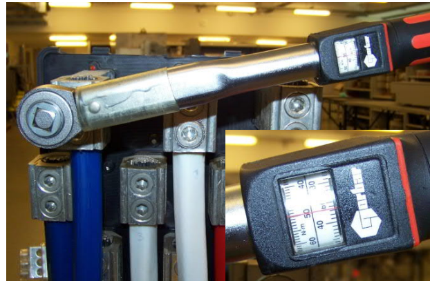
Figure 4: Torque wrench set at 50Nm used to tighten the connections. Note all screws finish flush with the housing when tightened correctly
