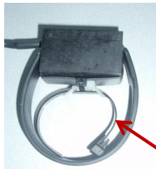
Figure 1- check cable tie
