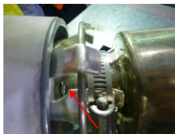
Figure 5 - Fuse (Fig 1) striker insufficient travel
