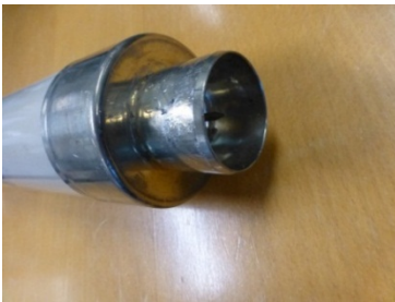
Figure 1 - Fuses with open end caps with striker
