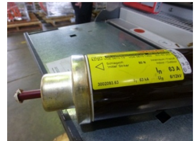
Figure 3 - Fuses with closed end caps with striker
