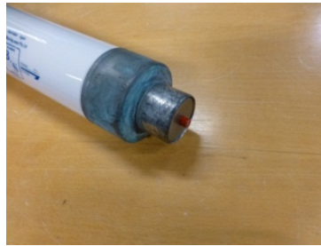
Figure 2 - Fuses with one end open, the other closed with striker
