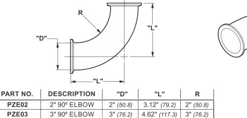
All fittings with standard Fab-Tech connections include gaskets and clamps or hardware as required for installation.
