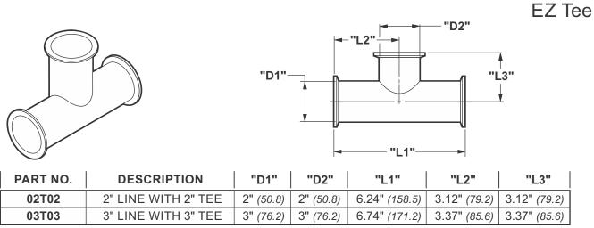
All fittings with standard Fab-Tech connections include gaskets and clamps or hardware as required for installation.
