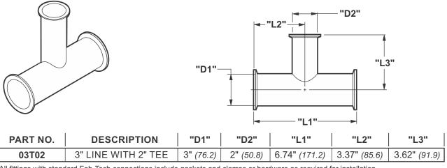
All fittings with standard Fab-Tech connections include gaskets and clamps or hardware as required for installation.
