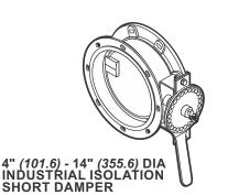
BODY: COATED 20GA (0.95) STAINLESS STEEL BODY LENGTH: 4" (101.6) MIN W/ EZ FLANGES 4-1/2" (114.3) MIN W/ CAST & FLAT RINGS **OPTION:** CUSTOM LENGTH COATING: PERMASHIELD FLUOROPOLYMER BARRIER COATING JOINING SYSTEM: FLOATING CAST STAINLESS STEEL RINGS **OPTION:** FLOATING STAINLESS STEEL
