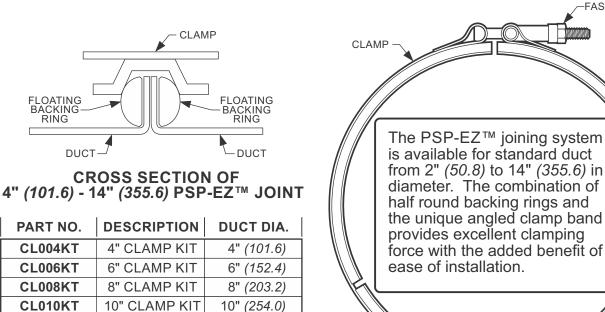
Each Kit above contains a clamp, PTFE tape gasket, and two backing rings
