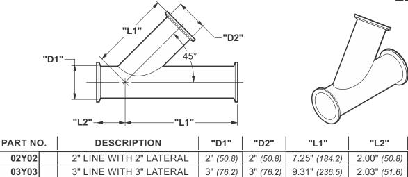
All fittings with standard Fab-Tech connections include gaskets and clamps or hardware as required for installation.
