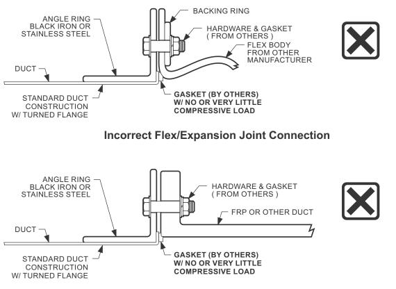
Incorrect FRP or Other Duct Joint Connection
