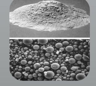
Generated by coal combustion. Composed of fine particles that are driven out of the boiler
