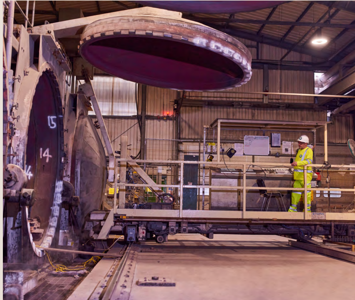
Operator preparing to unload finished blocks from the open autoclave.
