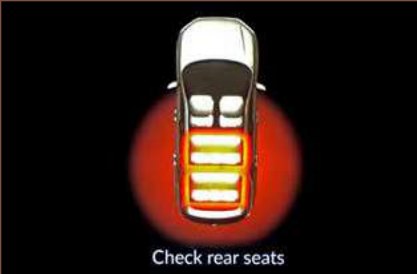
Rear Seat Reminder Rear Seat reminders system that you check the rear seat area, when the ignition is turned off.
