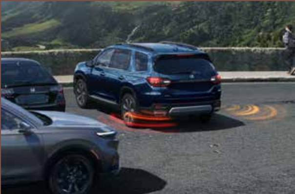
Rear Cross Traffic Monitor You can reverse out of a parking space with confidence, the RCTM provides an audible and a visual direction of the approaching vehicle on the audio screen.
