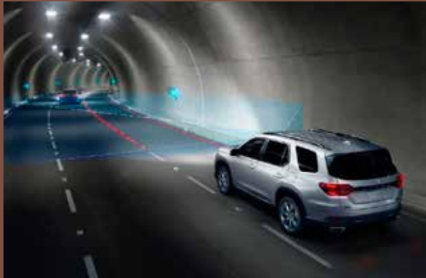
Auto High Beam Support The windshield mounted camera detects red and white lights of vehicles ahead. The system automatically switches the headlights from high to low beam, so you can concentrate on the road ahead.
