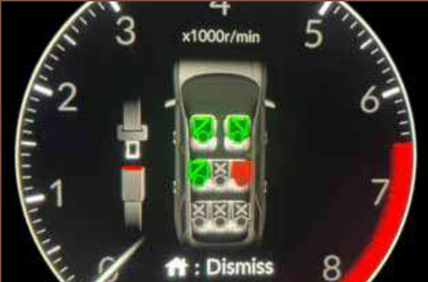
Seatbelt Reminder System Ensuring all occupants are belted up, a visual display is shown in the meter.
