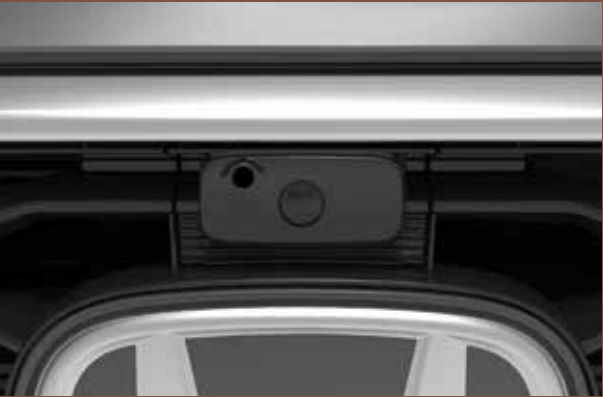
Front and rear cameras Front and rear cameras are equipped with washer nozzles, so you'll always get a clear picture of the surroundings.
