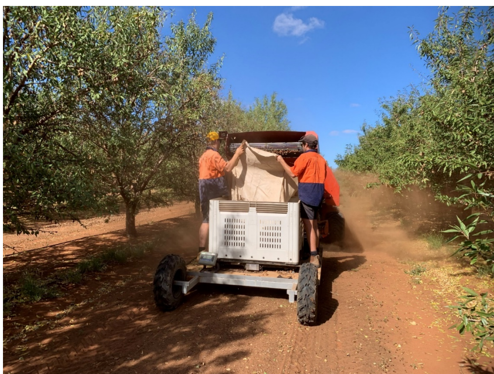
Figure B-1. A purpose-built trailer with scales attached behind a commercial almond harvester enabled more efficient pickup and weighing of fruit from trial plots.
