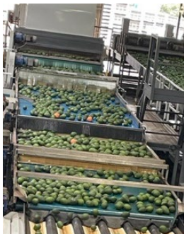
Image 1. Section of the CQ packing line (which included five drops) replaced in response to significant nodule damage noted in the 2023 DAF trial
