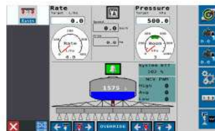
Figure 42: Activate pump control
