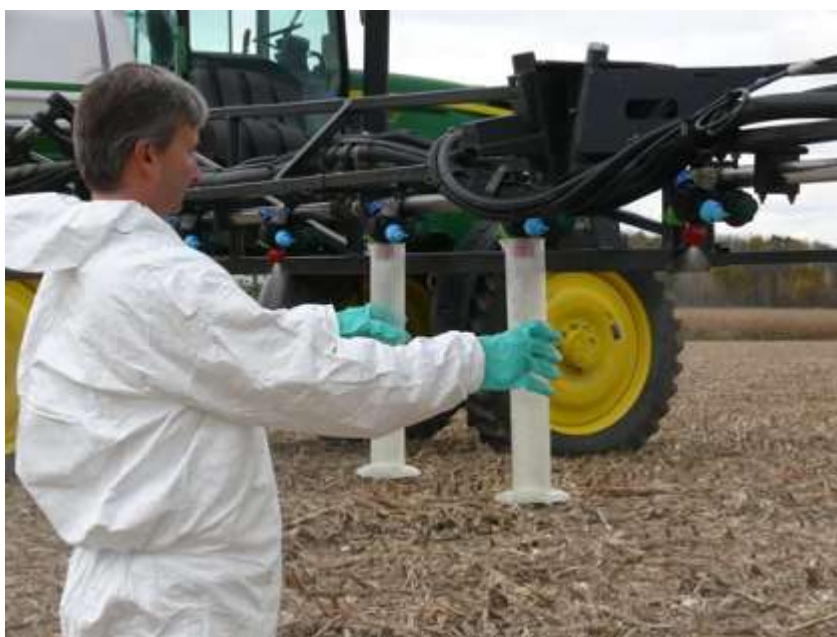
Figure 3. An Example of nozzle flow rate testing. source: https://sprayers101.com/
