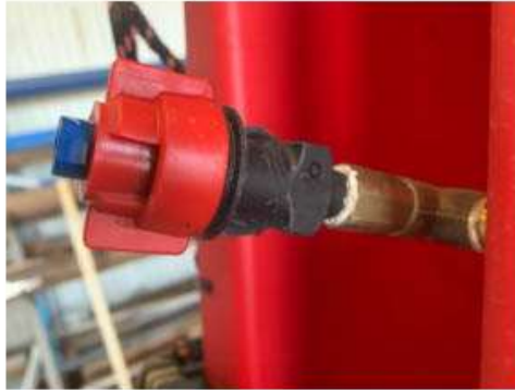
Figure 7: Assembled elbow, spacer, nozzle body and nozzle cap
