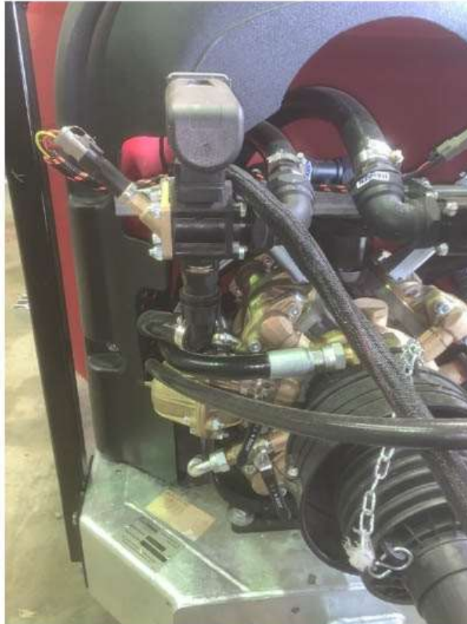
Figure 11: Boom control with Incorporated pressure transducer
