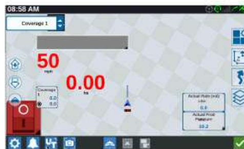
Figure 39: Main switch off
